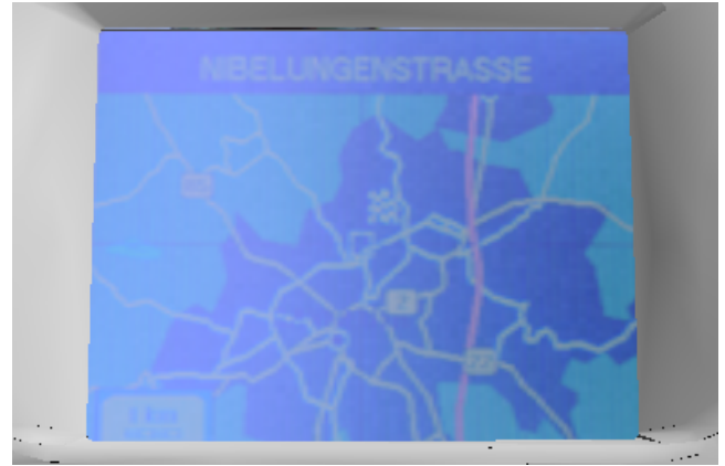
Figure 7: Converged image of the LCD panel. The image of this quality is shown after 2 seconds of computations by the cluster PCs.
