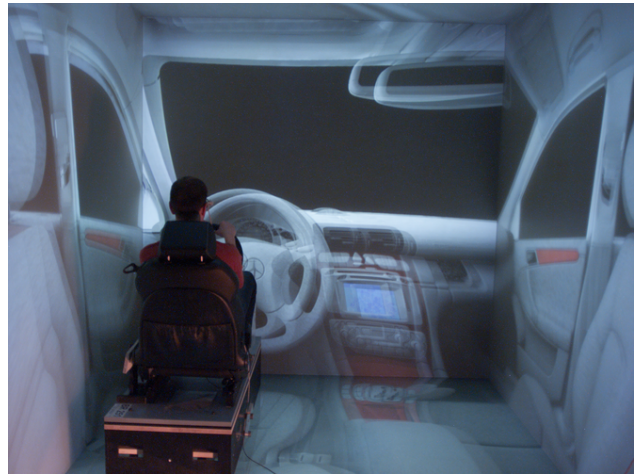
Figure 5: Interactive rendering of car interior. Photograph of the CAVE system with the stereo projection. The view is strongly distorted because it shows the car interior as seen from the perspective of the person wearing glasses with tracking device, but not the photocamera used to take this picture.
